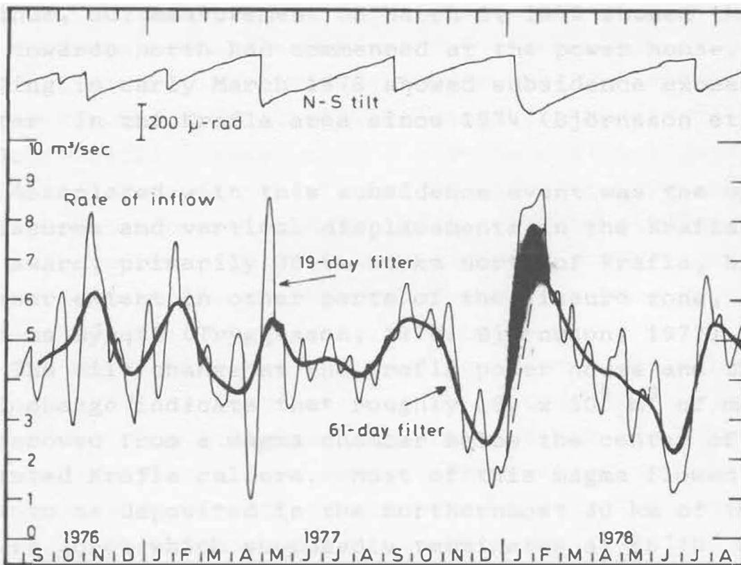
Fig. 3. The north component of tilt measured by the water tube tiltmeter in the Krafla power house (upper trace). Uplift to the north is up on the graph. The lower traces show the rate of tilt converted into rate of volume increase (inflow) of the Krafla magma chamber. This rate is filtered with a low pass filter to clarify the general trend. In January 1978 the inflow rate is uncertain due to prolonged subsidence event.
