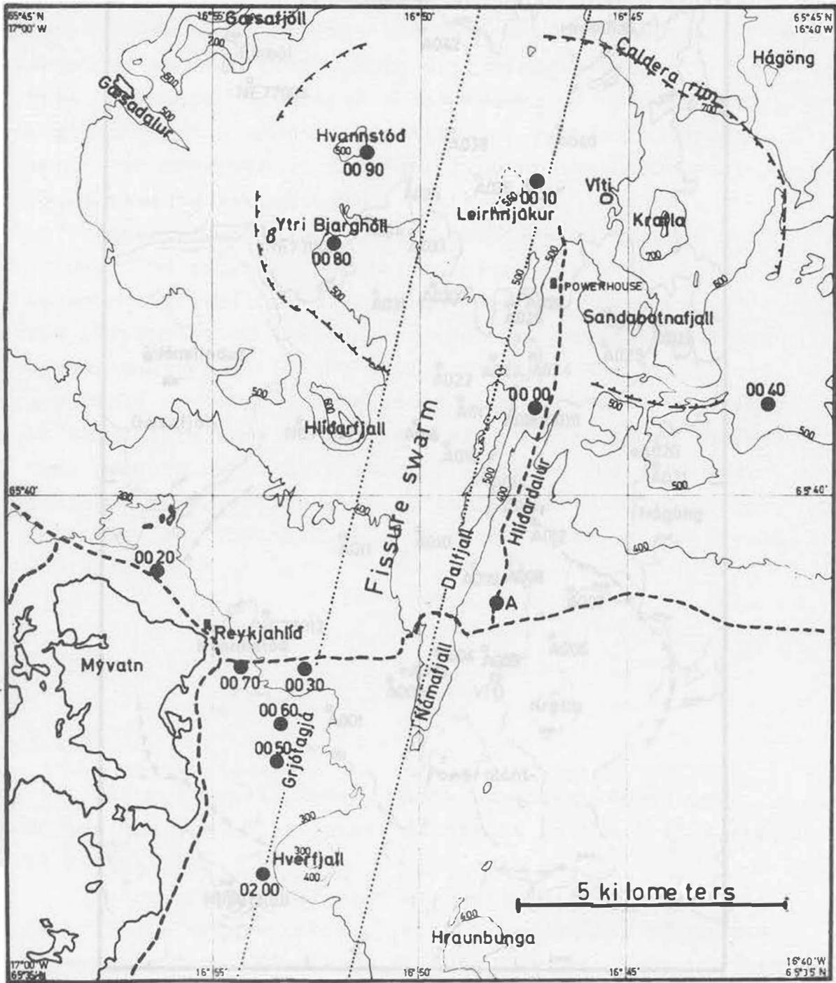
Fig. 1. Location of the spirit level tilt stations in the Krafla-Mývatn area (filled circles) and the electronic tilt-meters at the Krafla power house and Reynihlíð (near Reykjahlíð). The rim of the suggested Krafla caldera (Björnsson et al., 1977) is shown for reference on this and all subsequent maps.
