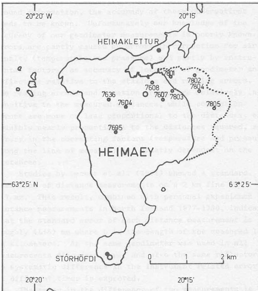
Fig. 2. The geodimeter network on the island of Heimaey Vestmannaeyjar (small circles). Also shown are the two stations, Heimaklettur and Stórhöfði, in the long distance geodimeter network (dots), and the two tiltmeter stations (open circles). The coast line before (solid line) and after (dotted line) the 1973 eruption is shown.
