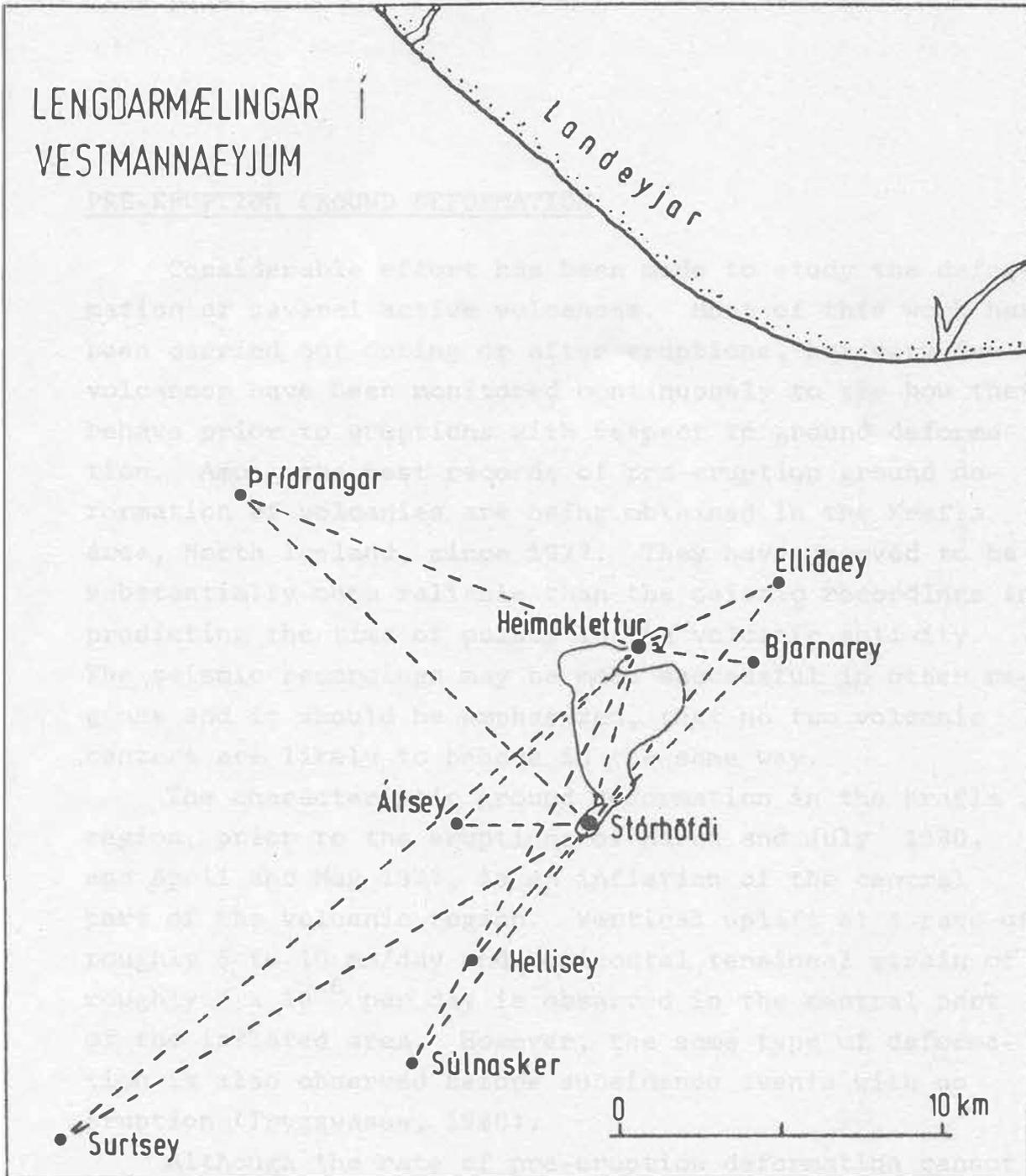
Fig. 1. The long distance geodimeter network in Vestmannaeyjar. North is up.
