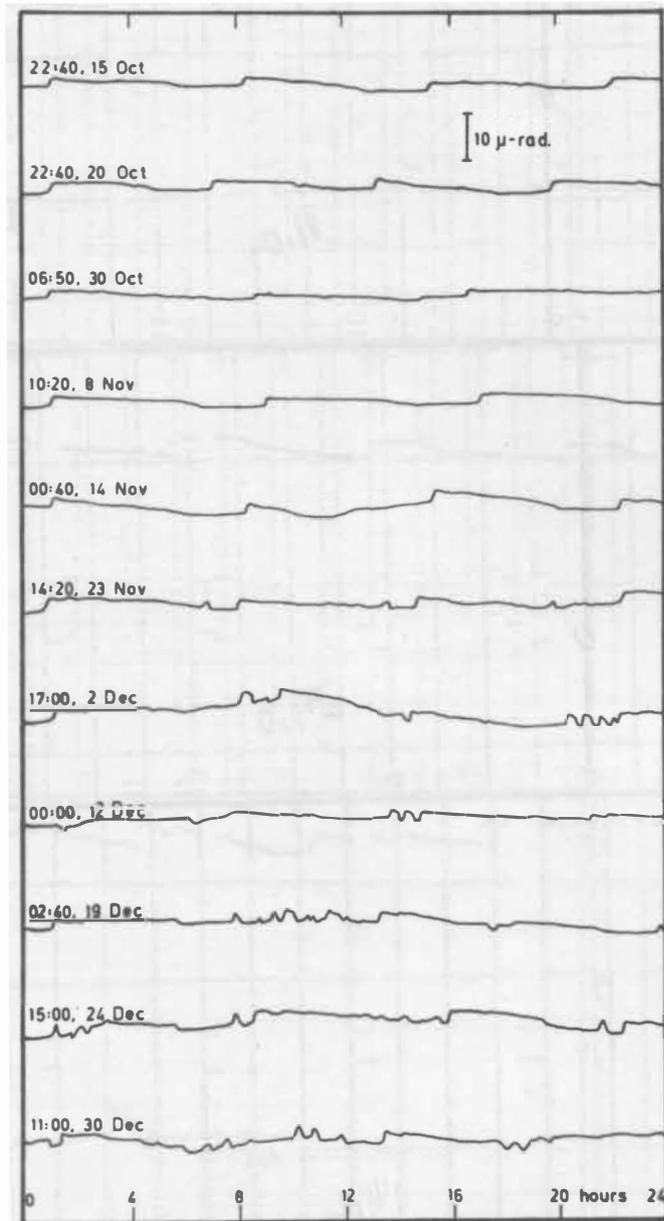
Fig. 15. Tracings of the N-component tiltmeter records at Litli Leirhnjúkur for 11 selected 24-hour intervals in 1980. The 7 hours periodic disturbance is especially clear on the 5 first records, but becomes less regular on later records.
