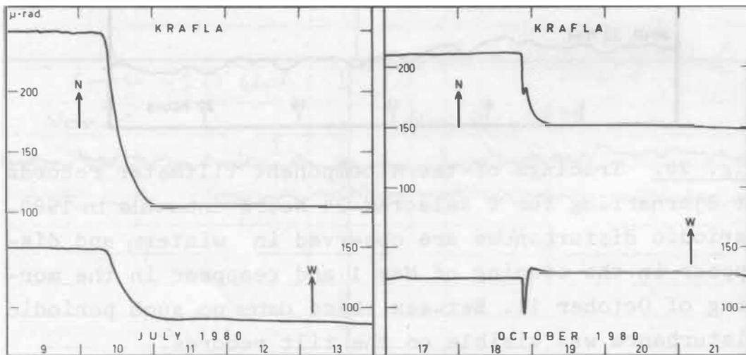
Fig. 21. Two subsidence events as recorded by the Krafla magnetoresistor tiltmeter. The reversal in tilt during the subsidence of October 18, is related to opening of ground fissures near the tiltmeter.
