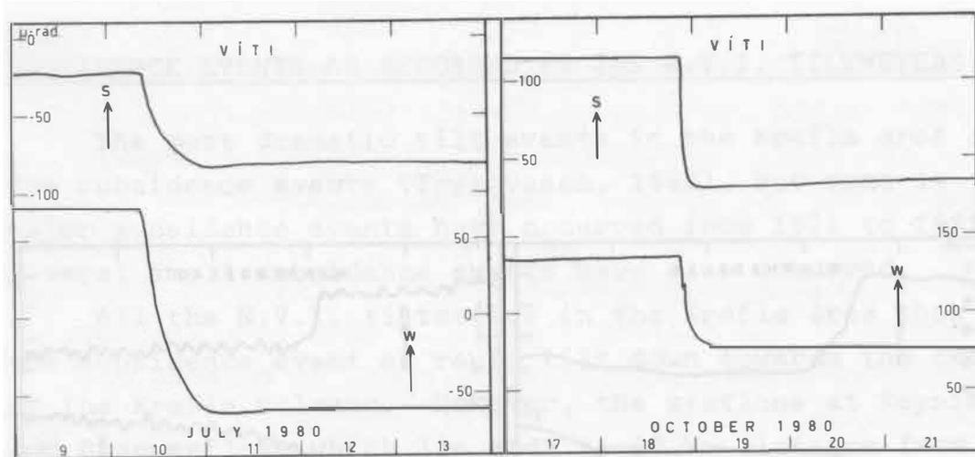
Fig. 22. Two subsidence events as recorded by the Viti tiltmeter.
