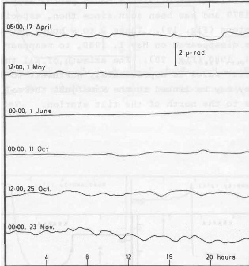
Fig. 20. Tracings of the N-component tiltmeter records at Bjarnarflag for 6 selected 24 hours intervals in 1980. Periodic disturbances are observed in winter and disappear in the evening of May 1 and reappear in the morning of October 11. Between these dates no such periodic disturbance was visible on the tilt records.
