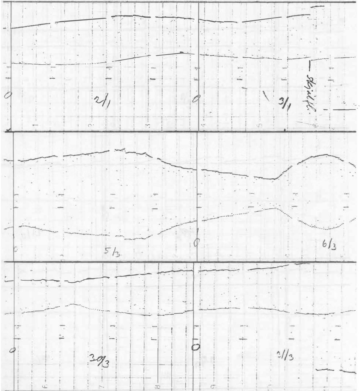
Fig. 12. Three 48 hours sections of tilt records from early 1980 in Litli Leirhnjúkur. The records are greatly disturbed by thermal strain, especially on March 5-6. Earthquake caused step in tilt record on January 3. The 90 min periodic disturbance is clearly visible on March 30-31, and also, but less clearly, on March 5-6.
