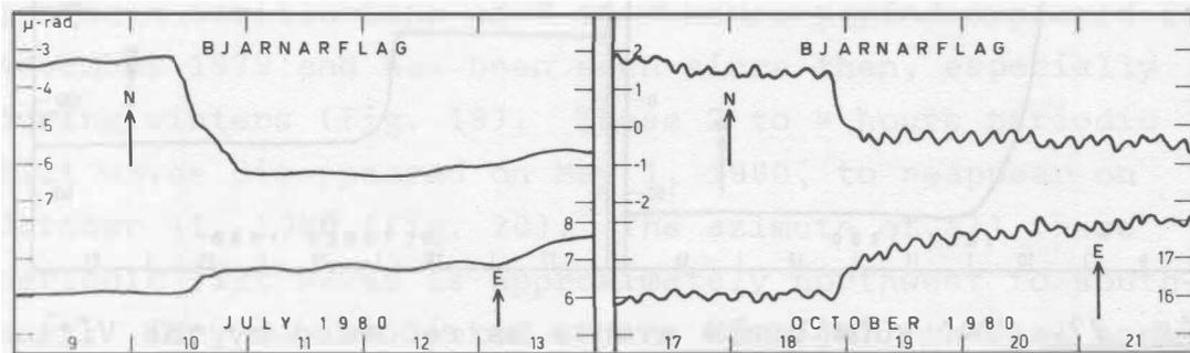
Fig. 24. Two subsidence events as recorded by the Bjarnarflag tiltmeter. Earth tide is visible on the July 9-13 records, but 3-5 hours periodic disturbance is very clear on the October 17-21 records.
