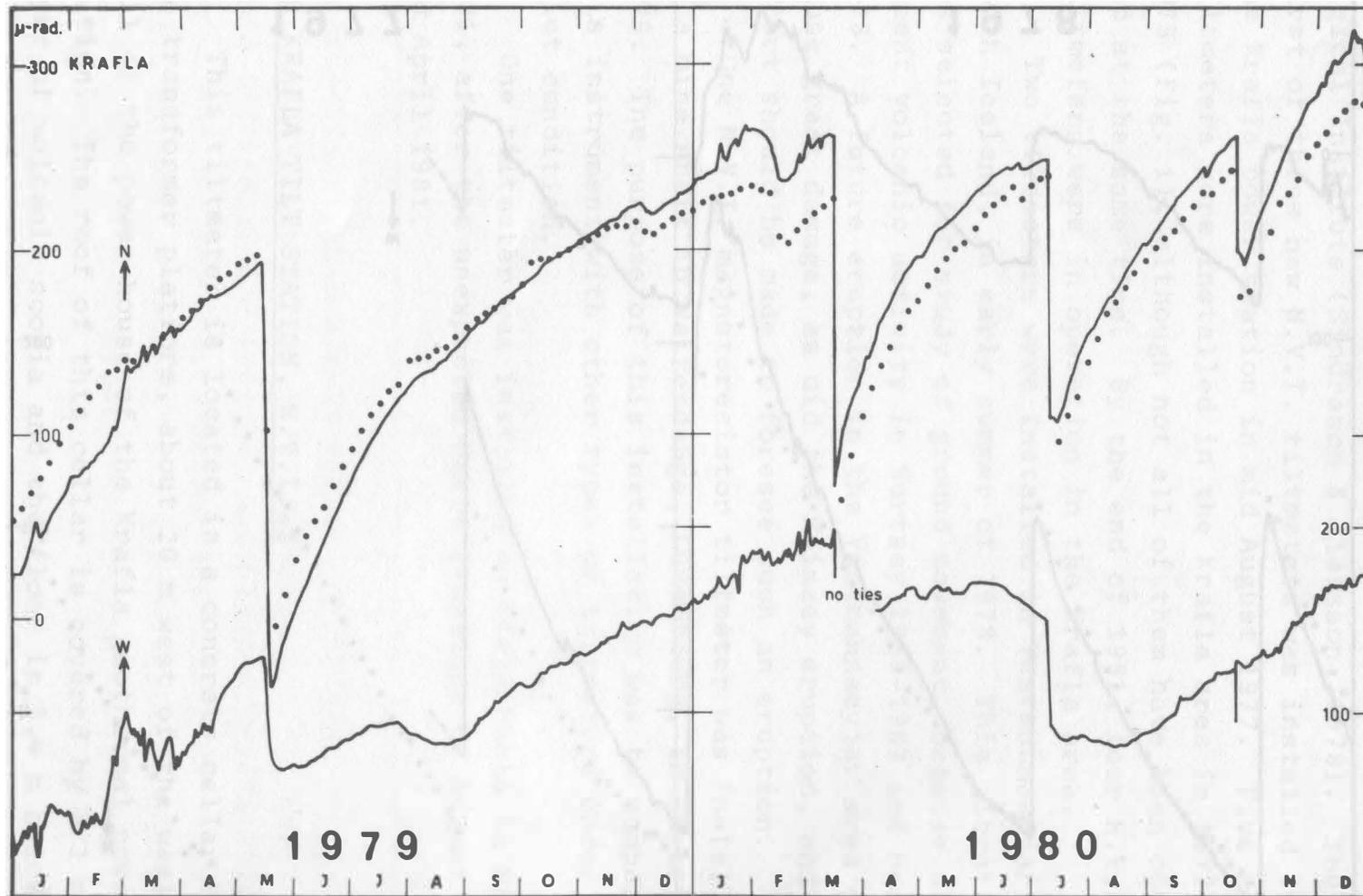
Fig. 3. Records of the Krafla tiltmeter 1979-1980. See Fig. 2 for explanation.
