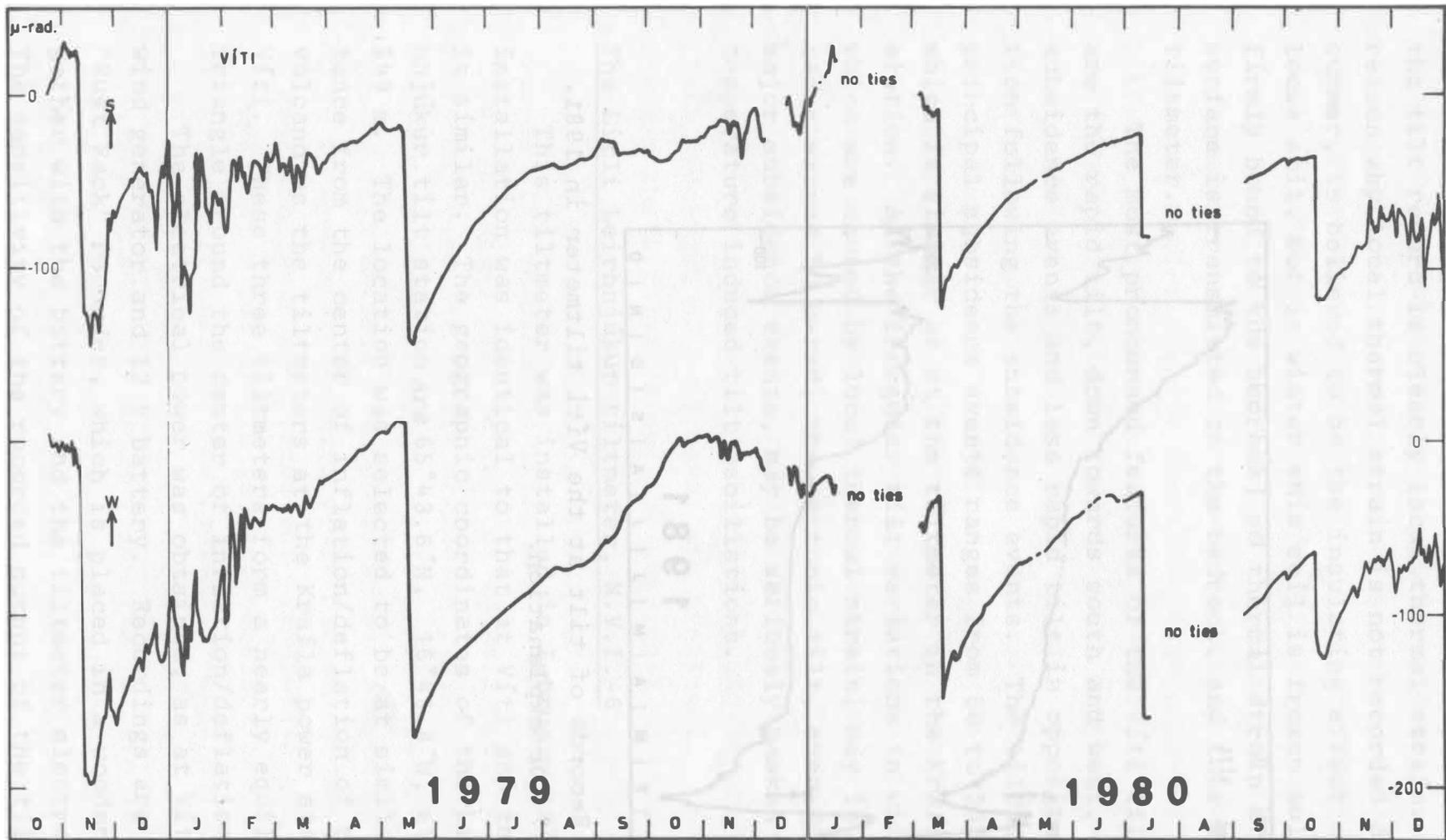
Fig. 7. Records of the Viti (N.V.I.-5) magnetoresistor tiltmeter, October 1978 to December 1980. The tilt stage in early March 1980 and early September 1980, are given arbitrary values after extended loss of records. Upper solid curve shows the N-S component of tilt, up is rising towards south (left scale). Lower curve is the E-W component of tilt, up is rising towards west (right scale).
