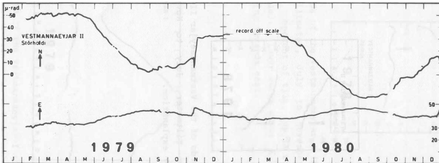
Fig. 28. Records of the Vestmannaeyjar II tiltmeter 1979-1980. The rapid tilt in mid November 1979 occurred during very heavy rainfall. See Fig. 25 for explanation.
