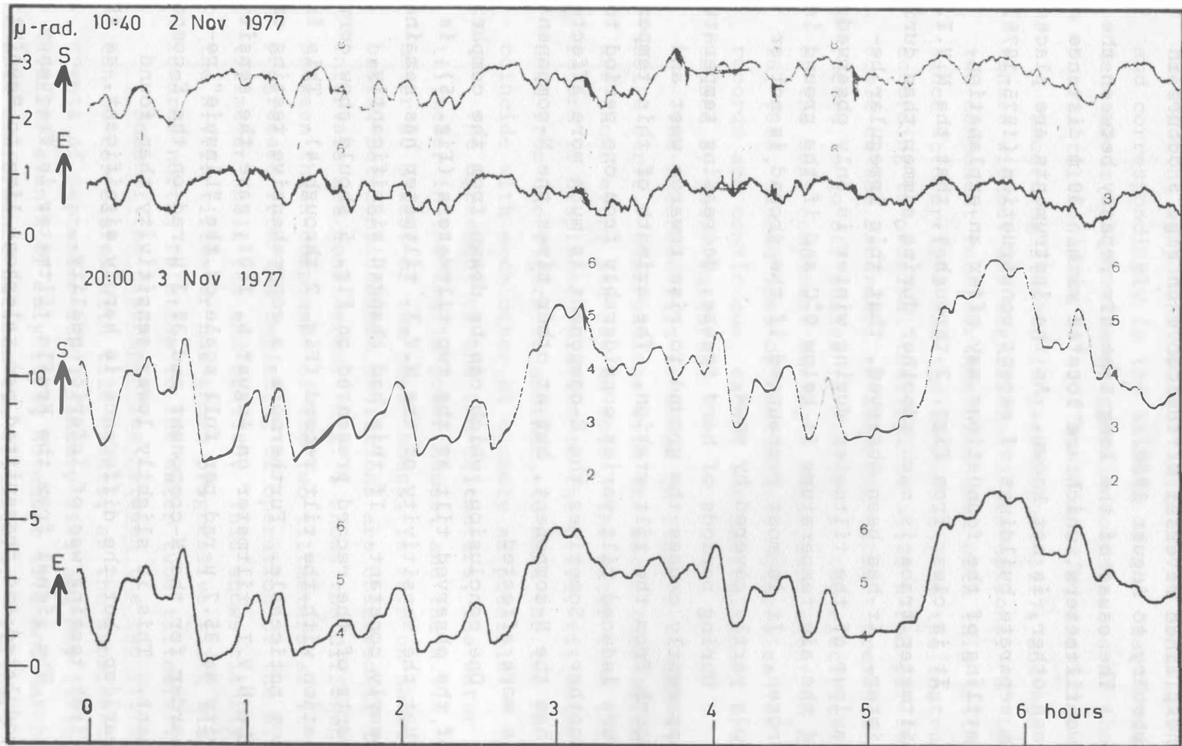
Fig. 6. Sample records of the Reynihlíð magnetoresistor tiltmeter. Arrows show direction of uplift. The unexplained irregular variations of apparent tilt have a stable azimuth of NW-SE.
