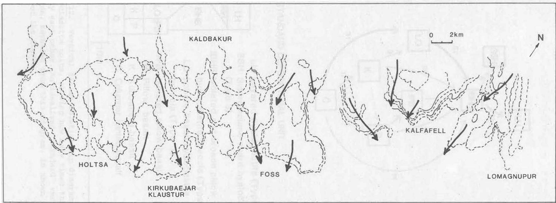
Fig. 11. Map showing axes of paleovalleys and main flow directions of the hyaloclastite units.
