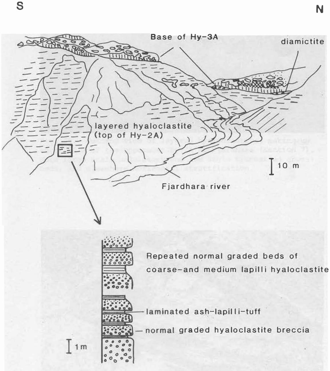
Fig. 24. Sketch of layered hyaloclastite (LH) at the top of Hy-2A at Fjardhara, Section 7. The internal structure and composition of individual layers are shown in detail below.
