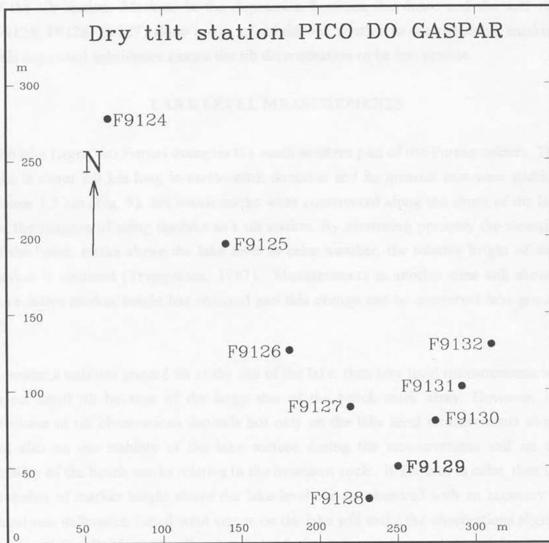
Fig. 4. Relative marker location of the dry tilt station Pico do Gaspar (solid dots). Marker F9129 is common for the two lines of levelling.
