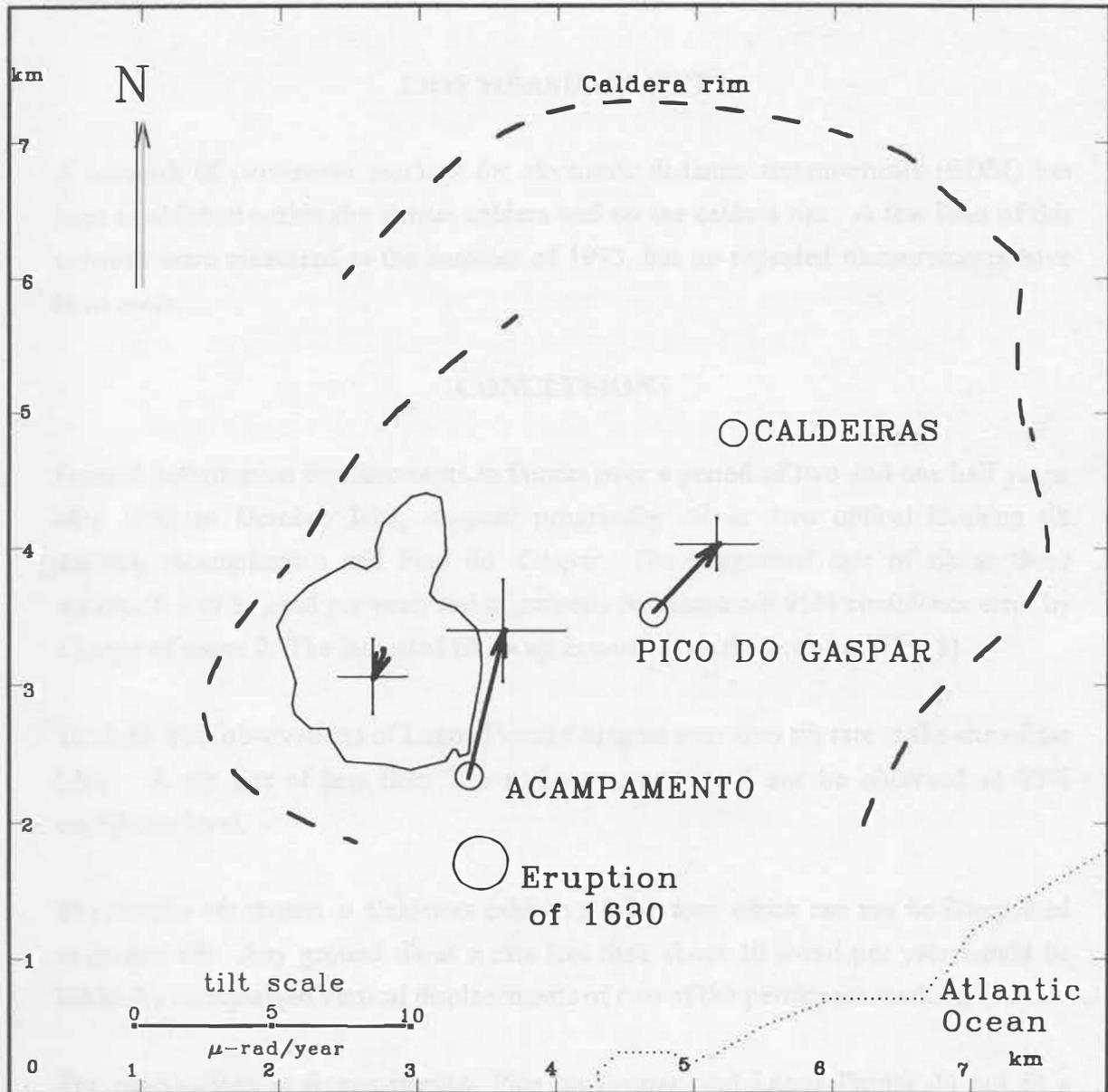
Fig. 8. Tilt rate at the dry tilt stations Acampamento and Pico do Gaspar, and at Lagoa das Furnas as derived from measurements of 1991 to 1993. Error bars show two times standard errors.
