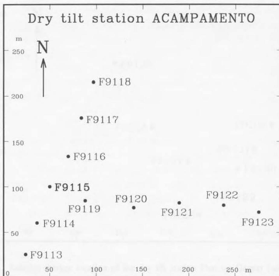
Fig. 3. Relative marker location of the dry tilt station Acampamento (solid dots). Marker F9115 is common for the two lines of levelling.
