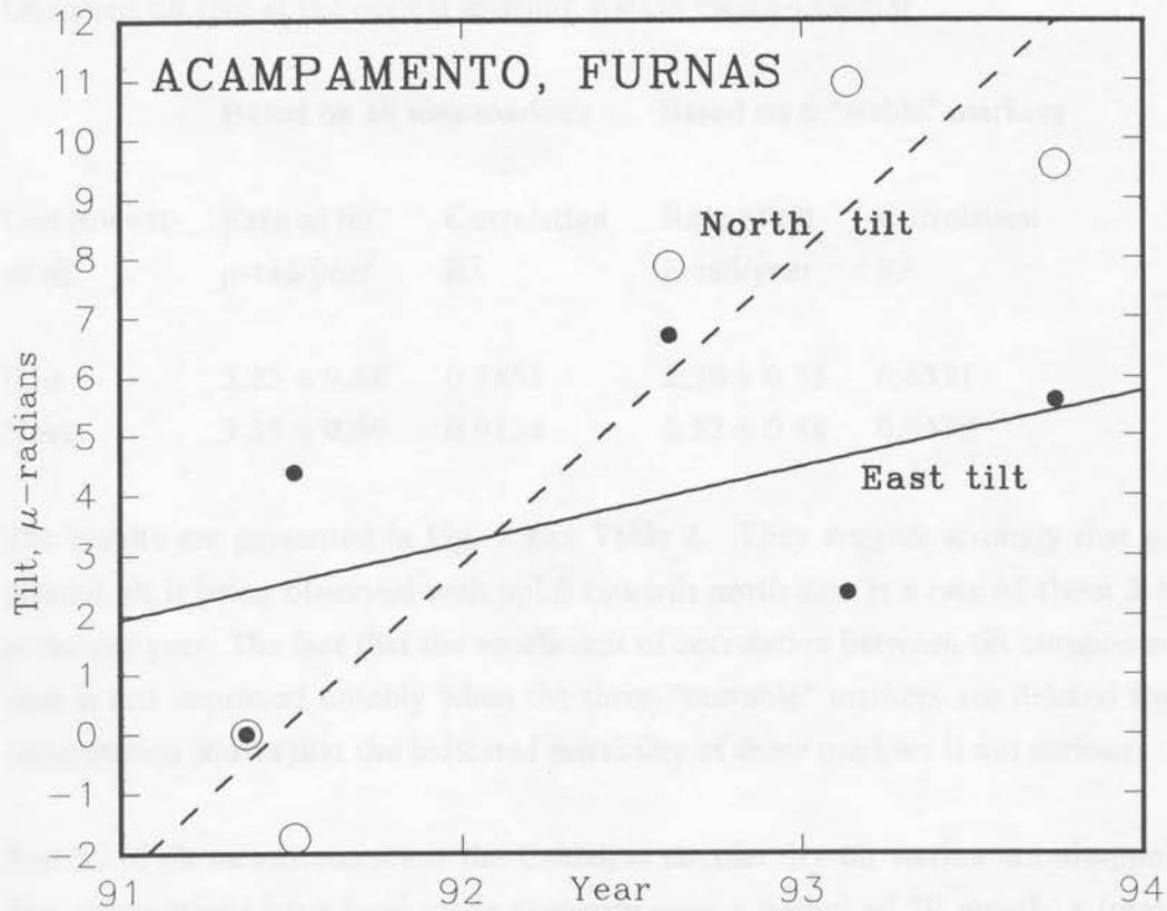
Fig. 6. Observed ground tilt at the dry tilt station Acampamento. Solid dots represent computed east component of tilt since first observation of May 1991 and solid line is the corresponding regression line. Open circles represent the north component of tilt and dashed line is the corresponding regression line. Positive tilt is uplift towards east and north.
