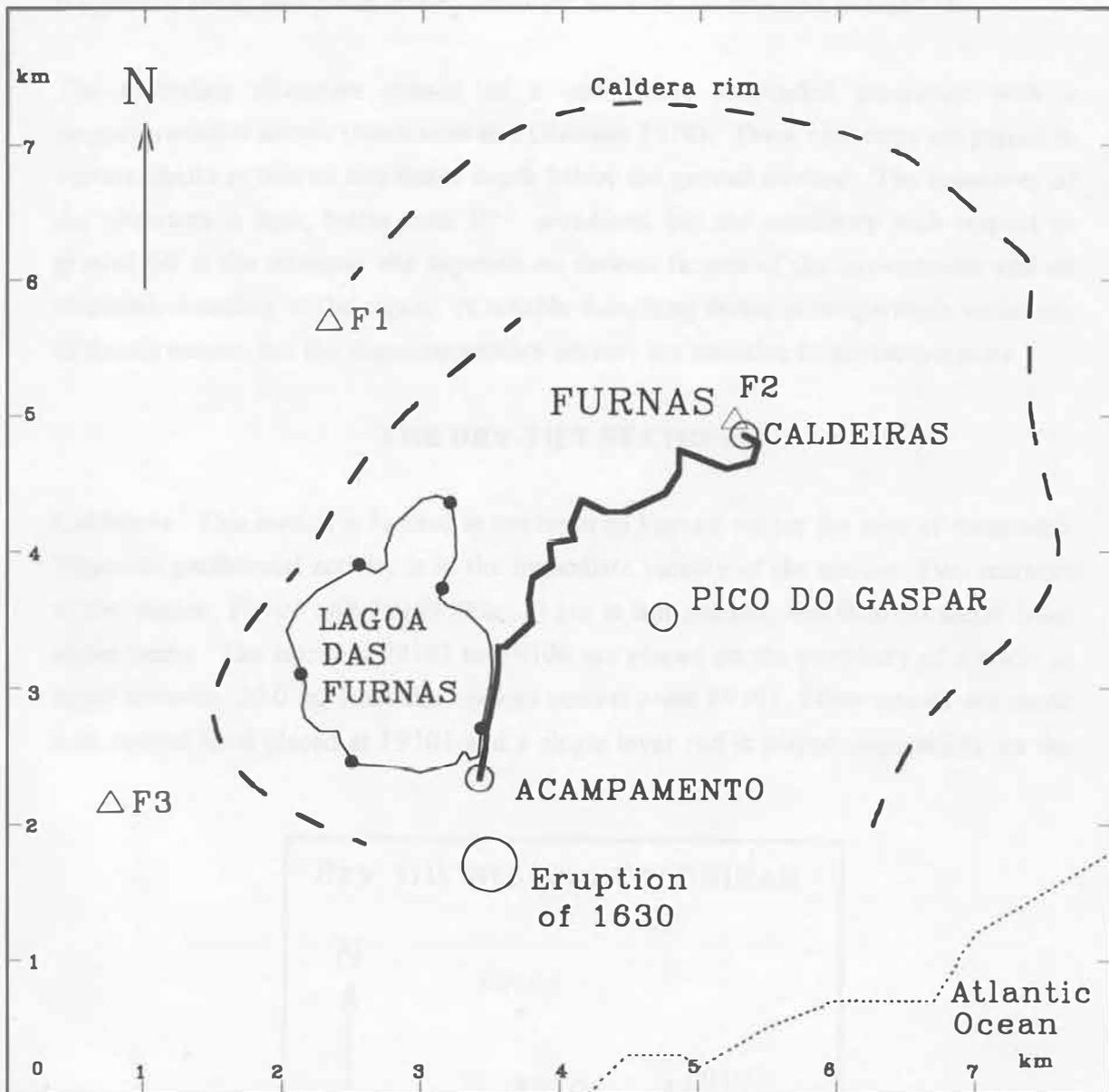
Fig. 1. Simplified map of the Furnas area showing dry tilt stations (small open circles), long levelling line (thick line), recording tiltmeters (open triangles), lake level stations (solid dots), the caldera rim (dashed line) and the site of the last eruption in the area (large open circle).
