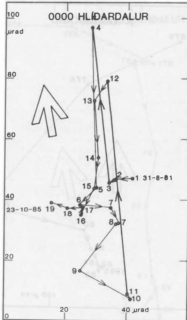
Fig. 6. Progressive tilt at the station 0000 based on single observations. See Fig. 3 for explanation.
