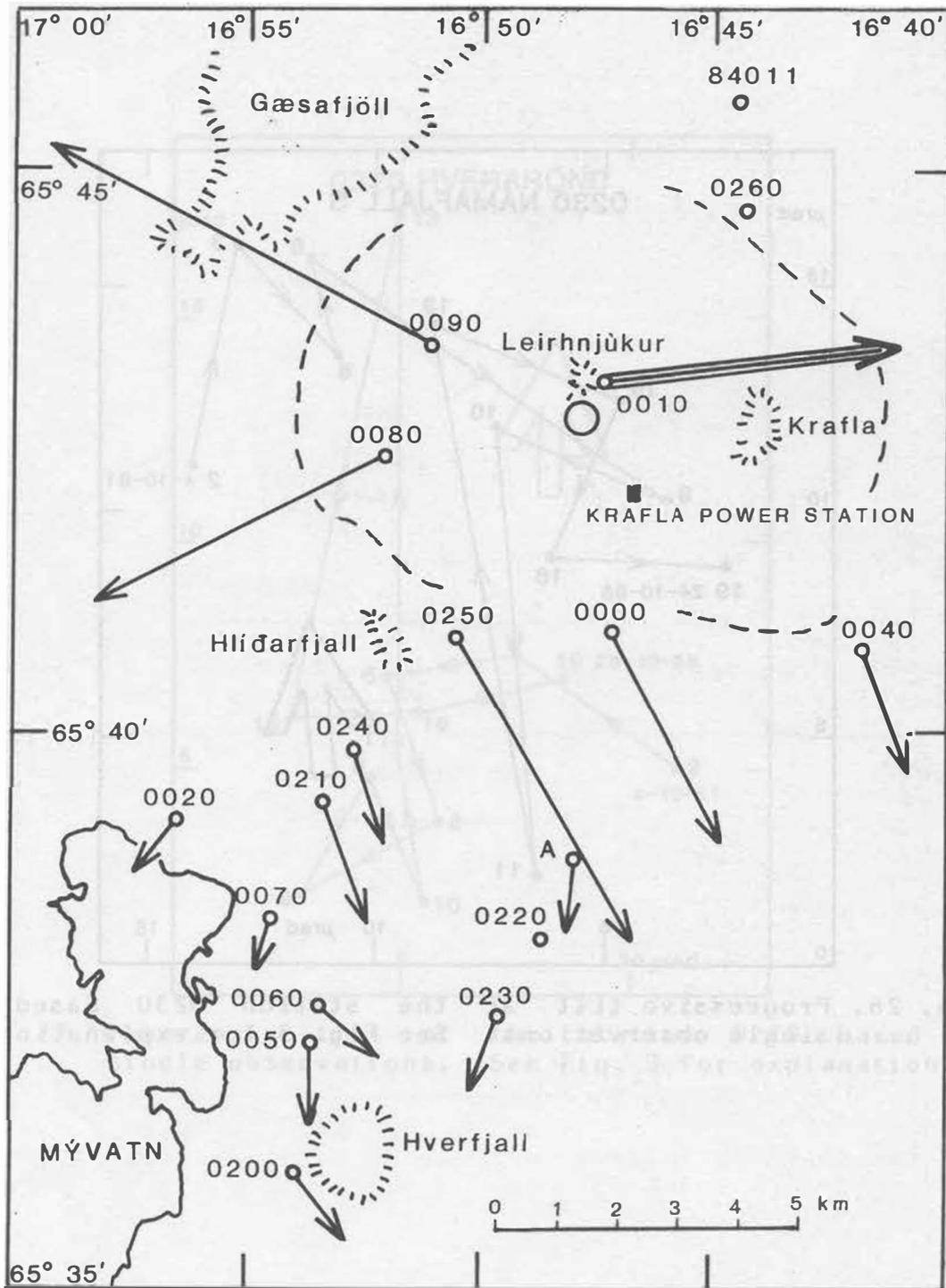
Fig. 29. Tilt during slow inflation of the Krafla volcano from May 1982 to June 1984. The arrow lengths are proportional to tilt except at station 0010 where the length of the arrow should be 4 times greater than shown.
