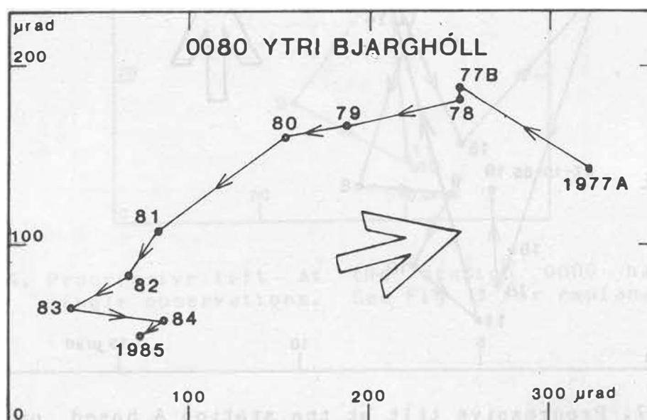
Fig. 9. Progressive tilt at the station 0080 on annual basis. See Fig. 2 for explanation.
