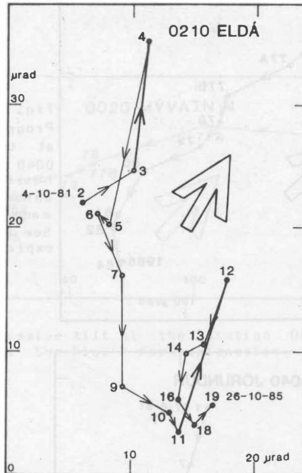
Fig. 14. Progressive tilt at the station 0210 based on single observations. See Fig. 3 for explanation.
