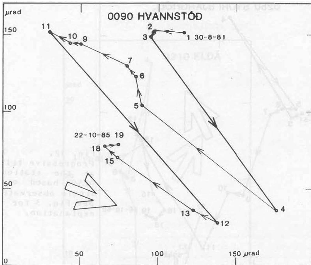
Fig. 10. Progressive tilt at the station 0090 based on single observations. See Fig. 3 for explanation.
