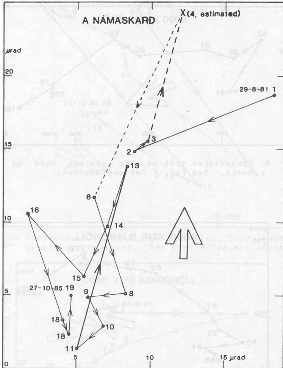
Fig. 7. Progressive tilt at the station A based on single observations. Tilt stage (4) is estimated at end of the November 1981 deflation. See Fig. 3 for explanation.
