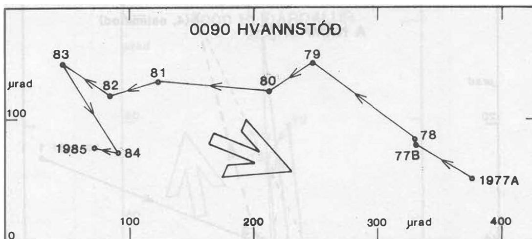
Fig. 8. Progressive tilt at the station 0090 on annual basis. See Fig. 2 for explanation.
