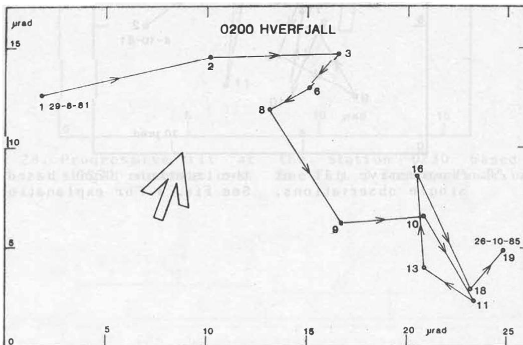
Fig. 26. Progressive tilt at the station 0200 based on single observations. See Fig. 3 for explanation.
