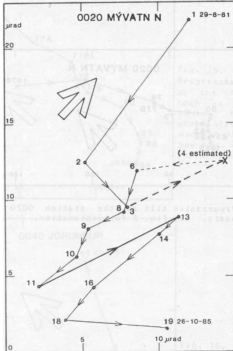
Fig. 18. Progressive tilt at the station 0020 based on single observations. See Fig. 3 for explanation.
