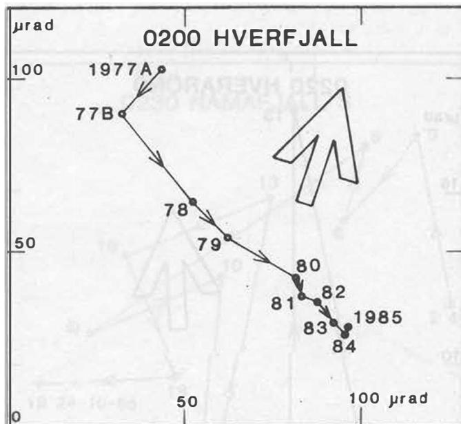
Fig. 25. Progressive tilt at the station 0200 on annual basis. See Fig. 2 for explanation.
