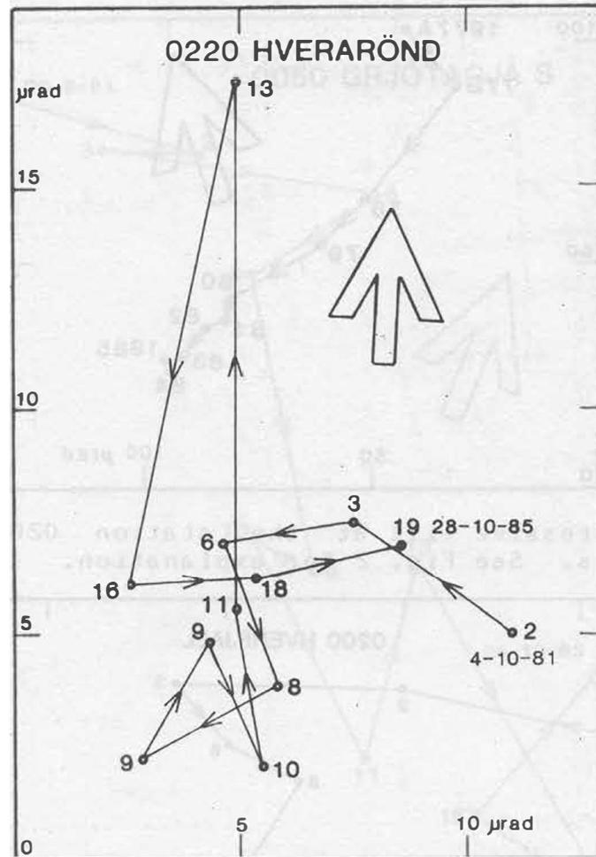
Fig. 27. Progressive tilt at the station 0220 based on single observations. See Fig. 3 for explanation.
