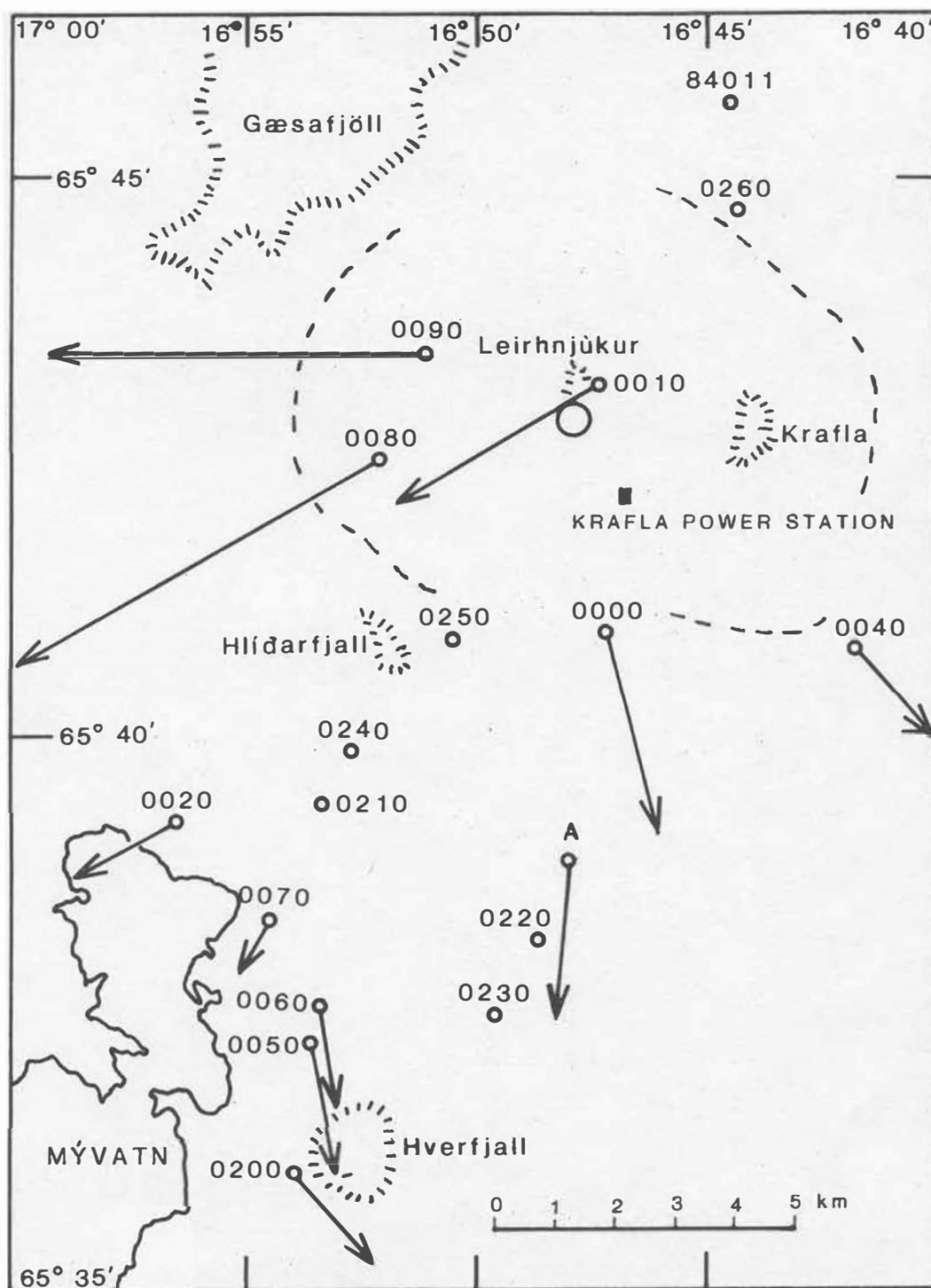
Fig. 30. Relative secular tilt at the optical leveling tilt stations in the Krafla-Mývatn area based on observations in 1979 and 1984. Station 0010 is anomalous because of extreme movement during several subsidence events, especially in March 1980.
