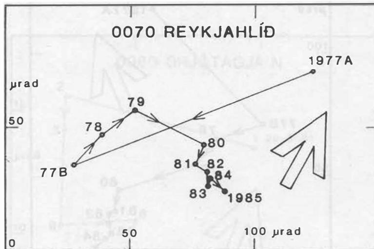
Fig. 19. Progressive tilt at the station 0070 on annual basis. See Fig. 2 for explanation.
