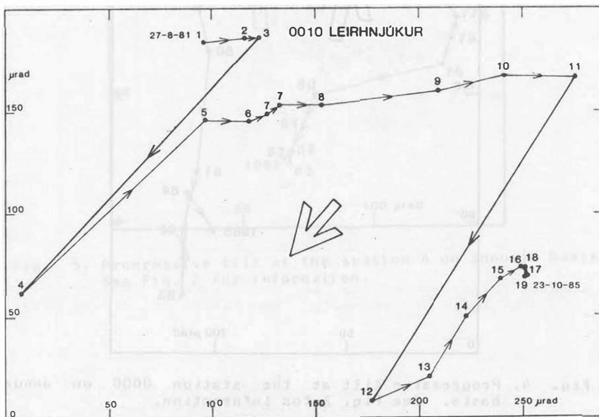
Fig. 3. Progressive tilt at the station 0010 August 1981 through October 1985. Data points show observed tilt stage at each tilt observation. Thick lines show tilt during deflation of Krafla. Numerals indicate times of observations as explained in the text. Date of first and last observation is given (dd-mm-yy). Large arrow shows direction to the center of inflation/deflation. See Fig. 1 for location of the station.
