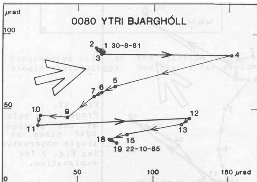
Fig. 11. Progressive tilt at the station 0080 based on single observations. See Fig. 3 for explanation.
