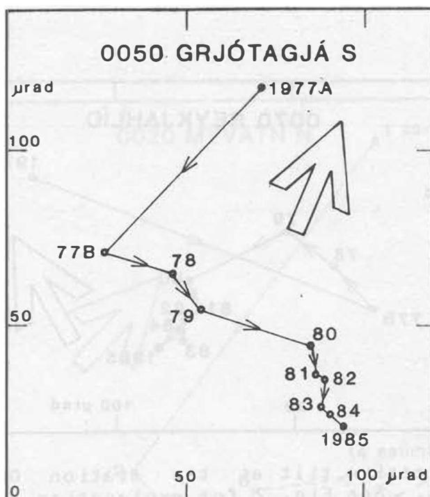
Fig. 21. Progressive tilt at the station 0050 on annual basis. See Fig. 2 for explanation.
