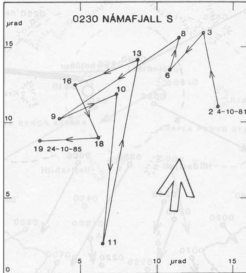
Fig. 28. Progressive tilt at the station 0230 based on single observations. See Fig. 3 for explanation.
