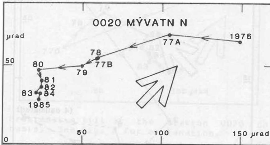
Fig. 17. Progressive tilt at the station 0020 on annual basis. See Fig. 2 for explanation.
