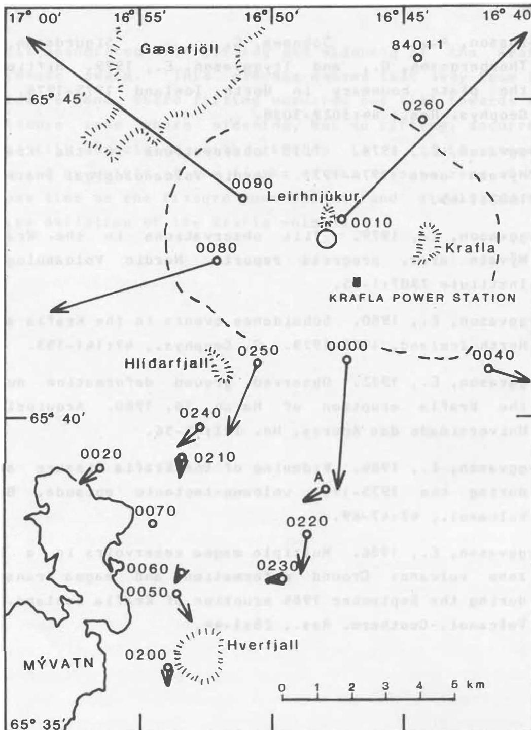
Fig. 1. Map showing the tilt stations in the Krafla-Mývatn area. Filled circles are recording tilt stations, open circles are optical level tilt stations. Two stations, 0260 and 84011 were established in October 1984 and are not included in the present discussion. Arrows show relative tilt from late September to beginning of December 1984. This is characteristic tilt during rapid inflation, following deflation of the volcano Krafla.
