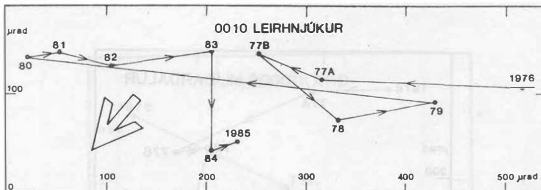
Fig. 2. Progressive tilt at the station 0010 from 1976-1985. Each data point gives average tilt stage of each year, although the year 1977 is split showing the average tilt stage before and after the September 8 deflation event. Large arrow shows direction to the center of inflation/deflation. See Fig. 1 for location of the station.
